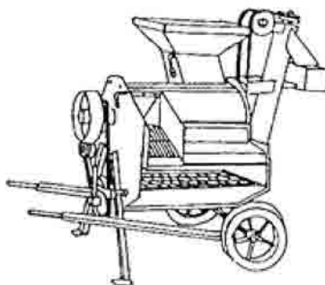
Fig. 1.7. Threshing, seed sorting, and grading equipment suitable for use on smallholder farms.
